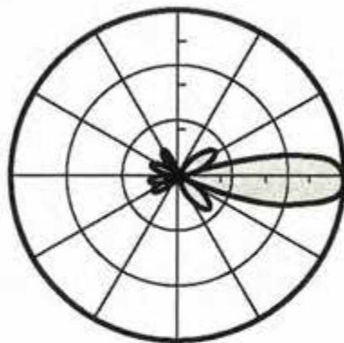
Fig. 6: Typical Narrow Beam-Width Aerial Radiation Pattern
